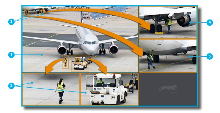
SeMSy<sup>®</sup> Compact Auto Tracking uses the VCA data of Dallmeier network cameras and Panomera<sup>®</sup> systems. While the video stream is displayed (live and playback), the analysis data allows the detection of image areas with moving persons or objects. These areas are displayed optimally zoomed in a detail split and ensure a targeted attention control during the evaluation.
