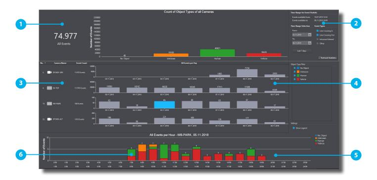
The SeMSy® Compact Dashboard displays the data of the event types Line Crossing, Intrusion Detection (image above) and Object Counting in a separate window as a bar chart. Besides a basic overview of all events, individual cameras can be selected for the evaluation of the recorded events during the course of the day. This view also supports the direct display of the corresponding recordings with the SmartFinder function.
