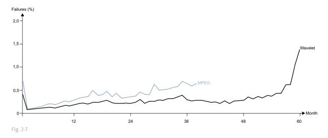
In contrast to the average MTTF of 550,000 hours specified by the manufacturer, an actually observed mean value (87% Wavelet with 247 000, 13% MPEG with 111,000 hours) of 220,00 hours was calculated. This corresponds to an actual observed AFR of about 3.9%.
