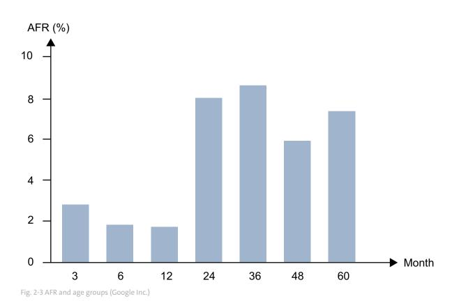
Fig. 2-4The **failure rate** was between 1.7% for HDDs that failed with an age of 1 year and 8.6% for HDDs that failed with an age of 3 years. The observed **AFRs are consistently much higher than the values provided by the manufacturer.**
