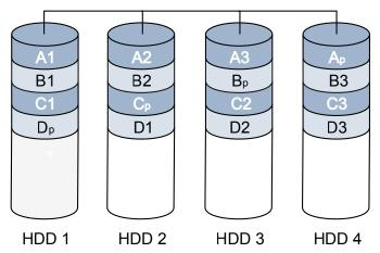
Fig. 3-3 RAID 5 with distributed data (e.g. A1 to A3) and parity data (e.g. Ap)
