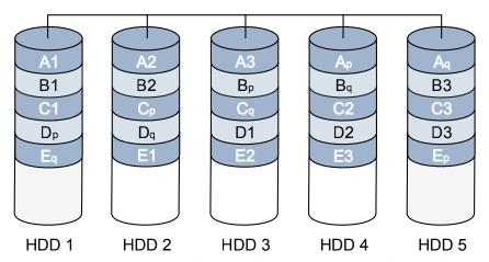
Fig. 3-4RAID 6 with distributed data (e.g. A1 to A3) and double parity data (e.g. 2 x Ap)
