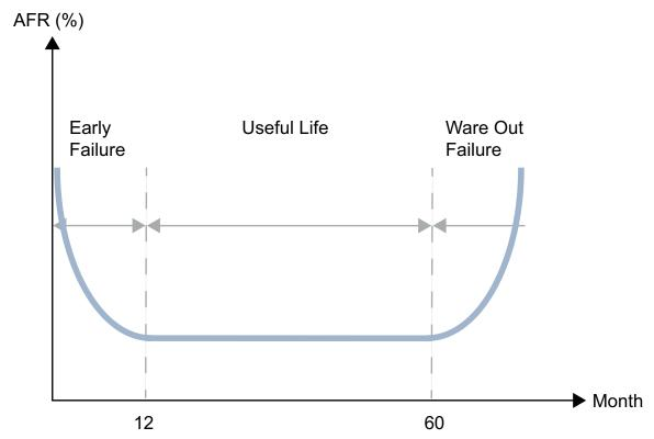
Fig. 2-5 Bathtub curve (theoretical model)
