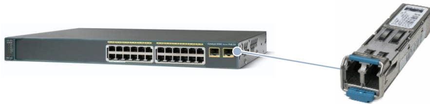
Fig. 2-3: Example of a SFP Interface with a matching module
