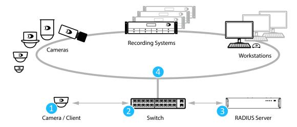
The camera is equipped with an individual certificate (ID card) before it is connected to the network.
