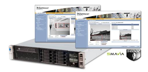
The **DVS 2500** is a SEDOR® video analysis server appliance for the analysis of up to 24 IP-based video streams. The dedicated server software **DVS Analysis Server** is installed ex factory and configured with a browser over Ethernet using the integrated **SEDOR® WebGUI**. Together with the optional licenses for the various **SEDOR® analysis applications** up to 24 channels can be used for video analysis according to demand.
