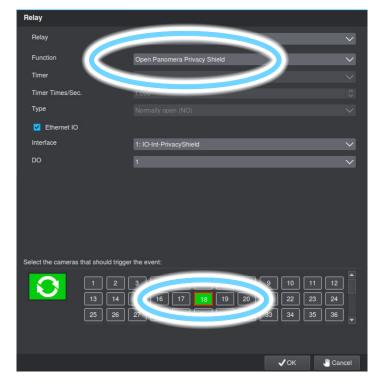
Both relays have to be assigned to the Panomera® Master Module, which in this example is recorded on channel 18.
