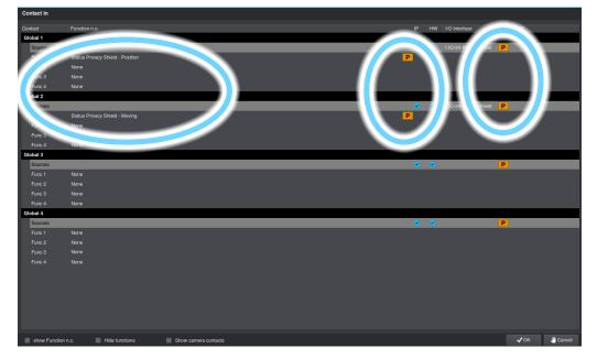
Subsequently, both contact functions (button **P**) must be assigned to the Panomera® Master Module, which in this example is recorded on channel 18.
