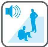
The **AI Loitering Detection App** analyzes the movement of persons detected by the neural networks and evaluates their dwell time in a defined sensitive zone. If the set limit value of the dwell time is exceeded, a corresponding message can be displayed to the operator. At the same time, undesired attendants can be requested to leave the area by outputting a stored audio sequence.
