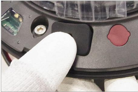
▶ Place the SD rubber seal back onto the recess and press it firmly into place with your finger.
