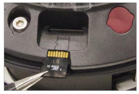
Use tweezers to insert the micro SD card. Pay attention to the orientation of the SD card as indicated on the embossing of the card slot.
