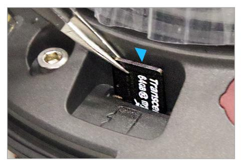
▶ Push the SD card completely into the slot by using tweezers and press it firmly until it clicks into place.
