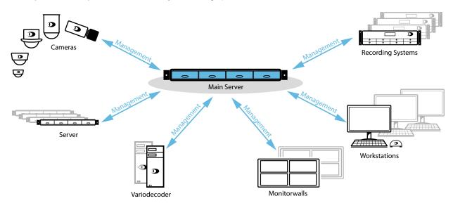
The HEMISPHERE® SeMSy® Main Server Software is the central management software for the entire SeMSy® Video Management System. The software manages all connections, streams, monitors and states of the complete system. All required configuration data (cameras, monitors, addresses, rights, priorities, etc.) is requested from the HEMISPHERE® SeMSy® Setup Server.
