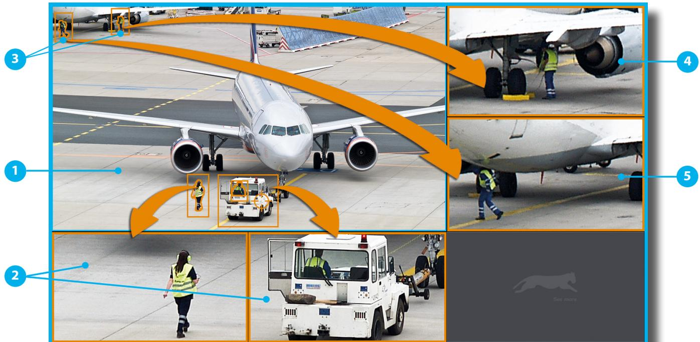
SeMSy® Compact Auto Tracking uses the VCA data of Dallmeier network cameras and Panomera® systems. While the video stream is displayed (live and playback), the analysis data allows the detection of image areas with moving persons or objects. These areas are displayed optimally zoomed in a detail split and ensure a targeted attention control during the evaluation.
