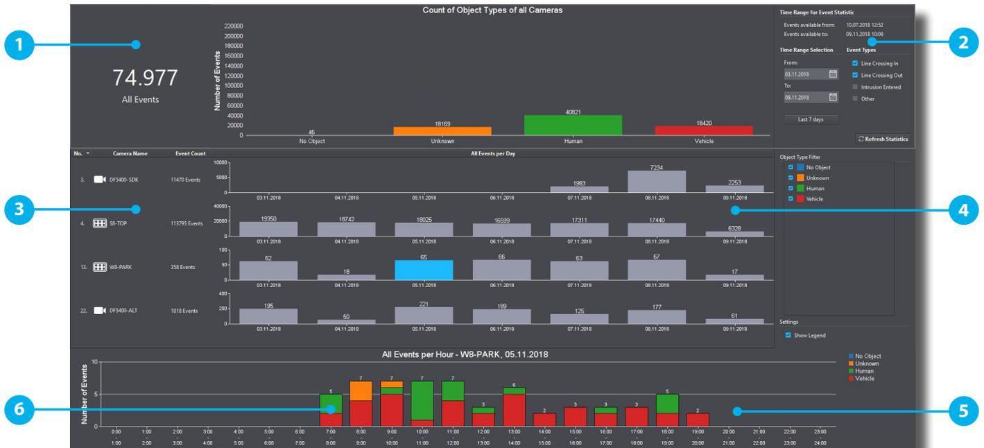
The SeMSy® Compact Dashboard displays the data of the event types Line Crossing, Intrusion Detection (image above) and Object Counting in a separate window as a bar chart. Besides a basic overview of all events, individual cameras can be selected for the evaluation of the recorded events during the course of the day. This view also supports the direct display of the corresponding recordings with the SmartFinder function.
