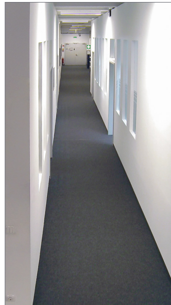
Full HD resolution, sensor aspect ratio 9:16, physical camera rotation of 90°, client-side image rotation of 90°
