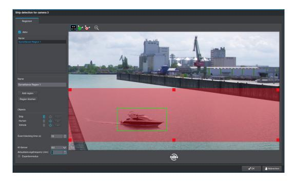
The SEDOR® AI Ship Detection software reliably detects large ships and small boats on open water areas, based on a powerful AI object classification with a specially trained neural network. The software analyzes the defined monitoring area in an adjustable cycle and immediately issues a corresponding message if a ship enters this area.
