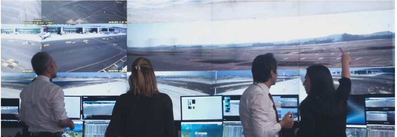
The “Virtual Tower” concept allows aircraft movements on the IGA to be tracked remotely.
