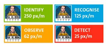
The standard DIN EN 62676-4 defines the required pixel densities depending on the application.
