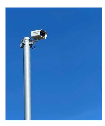
The patented Panomera® technology operates with optics having different focal lengths in one system. Therefore, a very small number of systems is sufficient to cover the large expanses of railway outdoor areas in high resolution.
