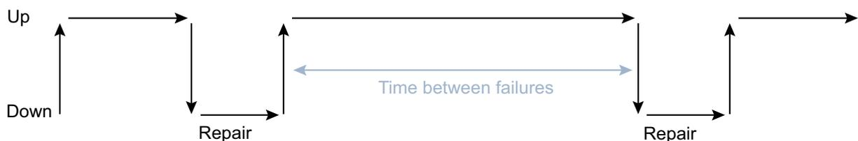
Fig. 2-1 MTBF - Time between failures
