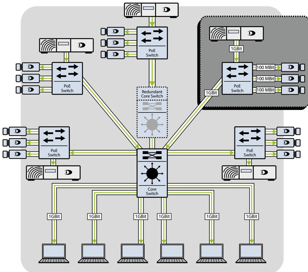
Fig. 3-7: “Large” Video Network (with a Star-Shaped Structure and Due To Multicast High-Performance)
