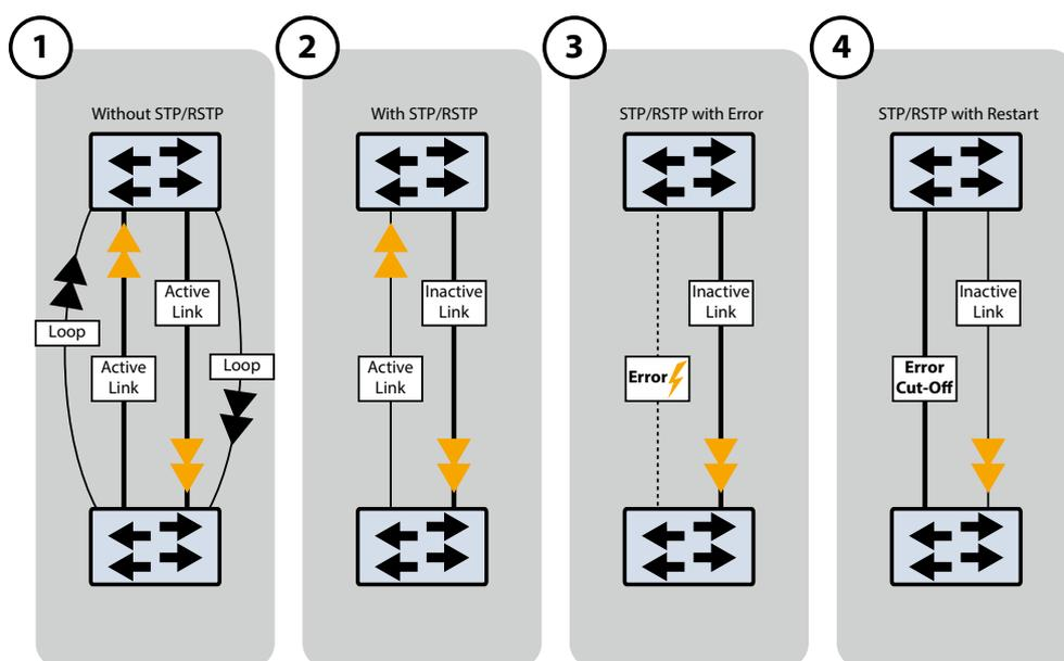
: STP (Spanning Tree Protocol) and RSTP (Rapid Spanning Tree Protocol)
