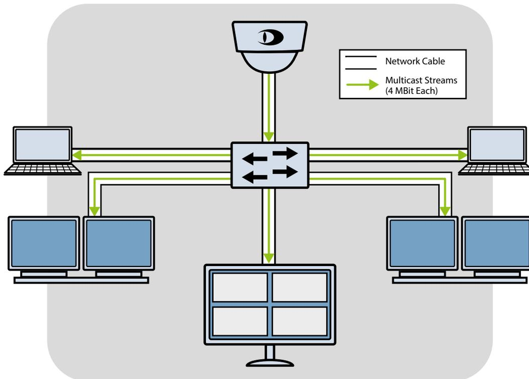
Fig. 3-2: Example for Video Streaming to a Multicast Group (IGMP V1)
