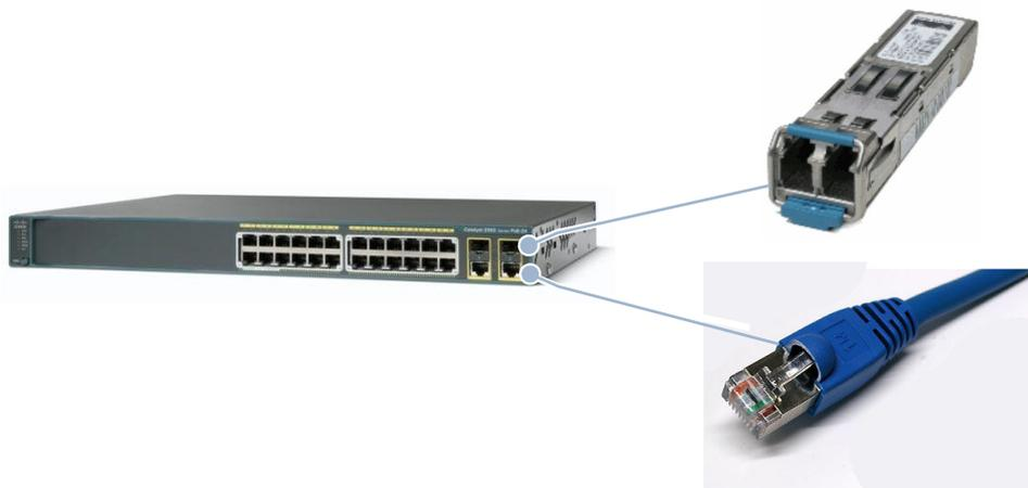
: Example Picture for a Dual-Purpose Interface with the Suitable Module and a RJ45 Connector with the According Jack
