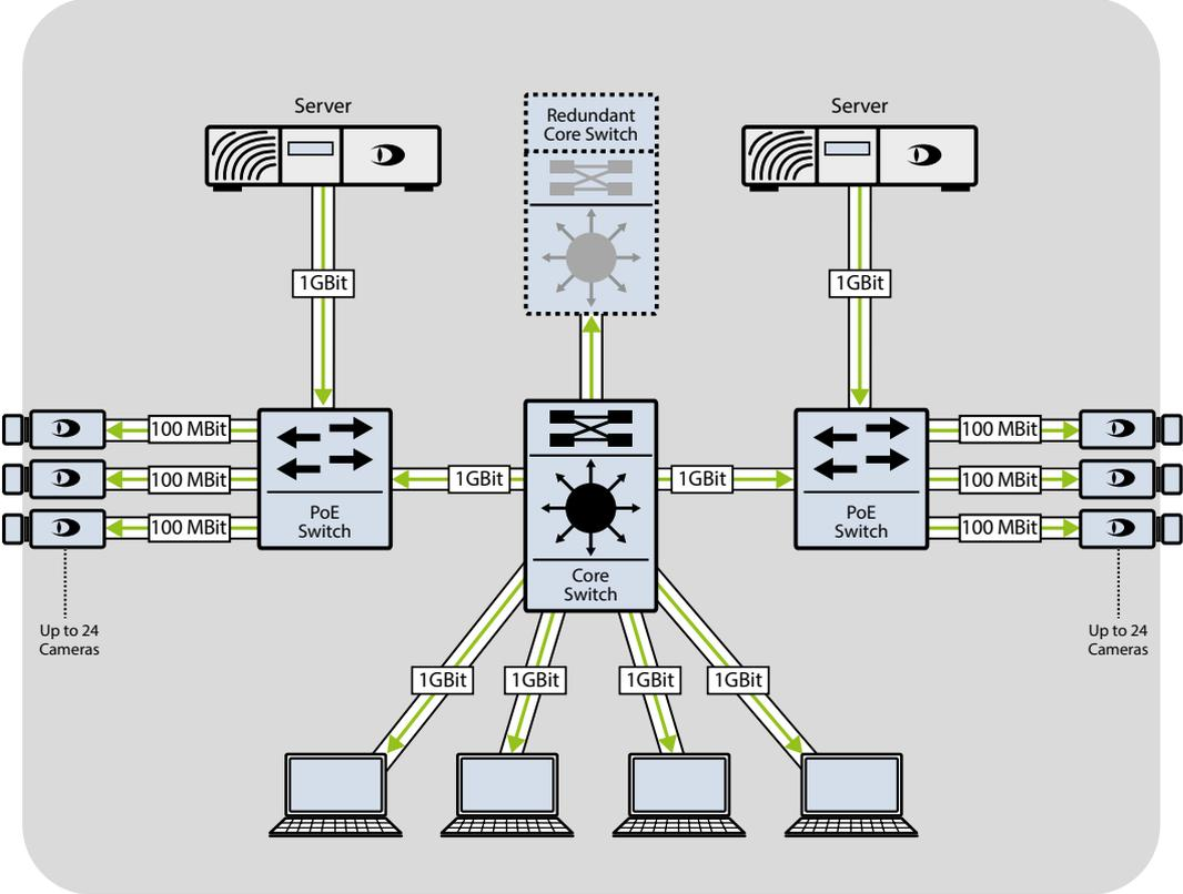
Fig. 3-6: Middle-Size Network with Core Switch (Optionally, a Further Redundant Core Switch)
