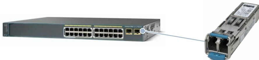
: Example Picture of a SFP Interface with the Matching Module
